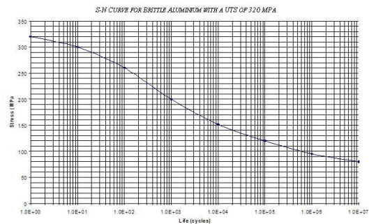
Figure 4 Experimental results for the life time of fatigue test samples (S-N curve), Photo from Wikimedia
