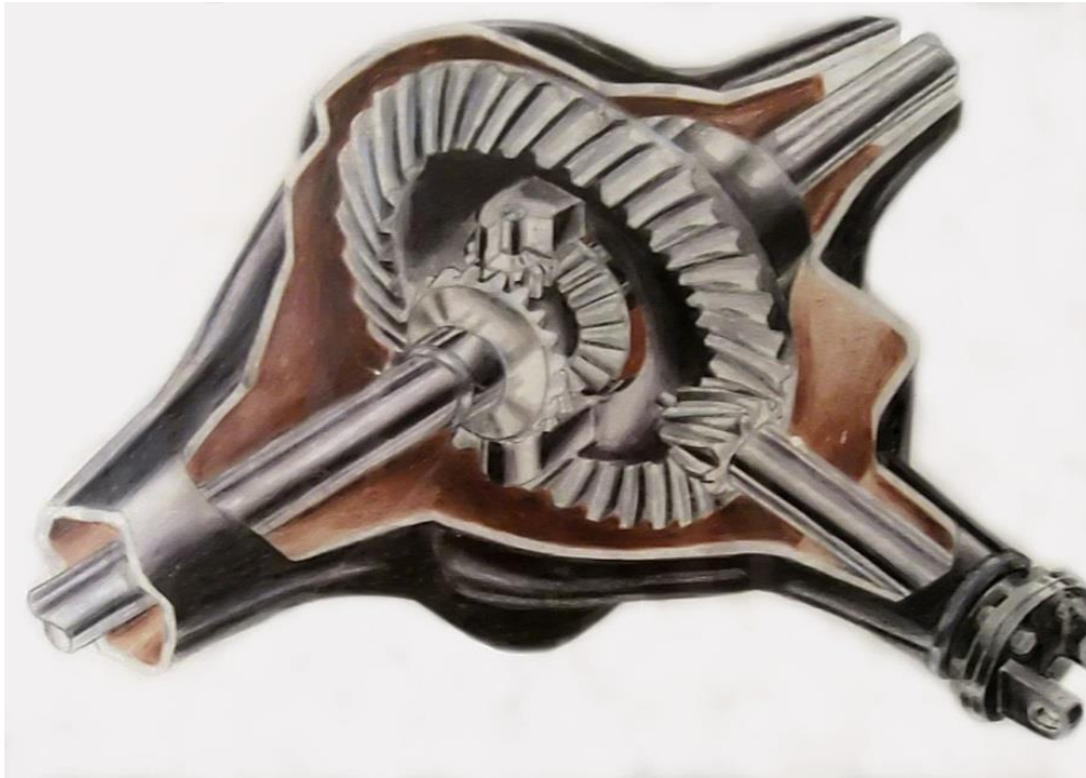
Figure 3-2 Shafts and differential for transmission of torque (from Wikimedia , GNU free documentation license)
